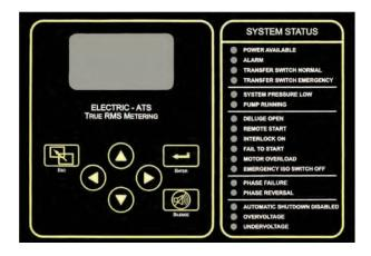
**Description**—Firetrol\* FTA1500 Primary Resistance Fire Pump Controllers use resistors in the line to reduce line voltage when starting the pump motor. The controller monitors, displays and records fire pump system information.
